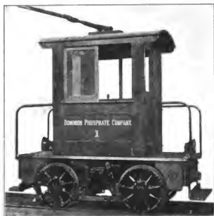
Fig. 4669. Baldwin-Westinghouse Electric Locomotive for the Dominion Phosphate Co. Weight, 12,000 lbs.; Diameter of Drivers, 30 in.; Wheel Base, 5 ft.; Drawbar Pull, Starting, 2,400 lbs.; Drawbar Pull, Running, 1,300 lbs.; No. of Motors, 2.
